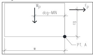
$x = \boxed{\begin{array}{c} \textbf{34.00} \\ \textbf{in.} \end{array}} \text{in.}$  x = lesser of L or W  $\text{dcg - Min} = \boxed{\begin{array}{c} \textbf{16.3} \\ \textbf{in.} \end{array}} \text{in.}$
